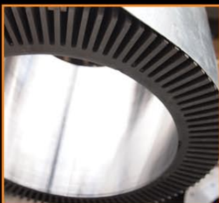
A water or air cooled heat sink can be fitted in the stator
